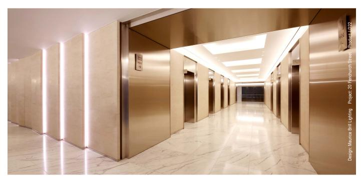
LD22 is a very small, low profile linear system. Designed to maximise the light output with a broad beam, it is ideal for coves, shelf details, recesses and highlighting architectural details. It is a 24V DC system allowing long lengths to be powered from a single driver.
